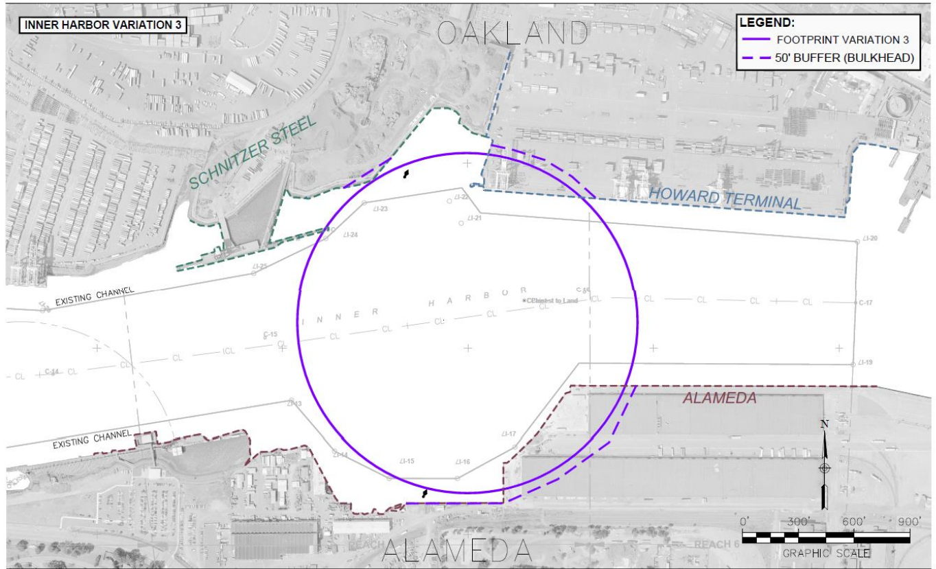
Figure 1: Proposed Inner Harbor Turning Basin Structural Features
